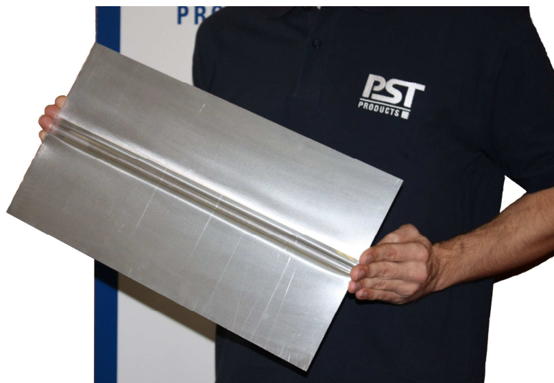
Fig. 7: EMPT welded samples of dissimilar metals respectively high wall thickness gradients (25.11.2010).
