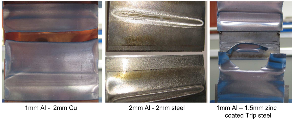
Fig. 5: EMPT welded tensile test specimen (25.11.2010)
